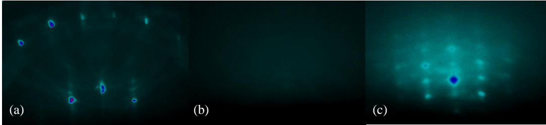
Figure 33: RHEED pattern of (a) sapphire substrate, (b) In DE, and (c) the nitridated QDs at 400 °C.
