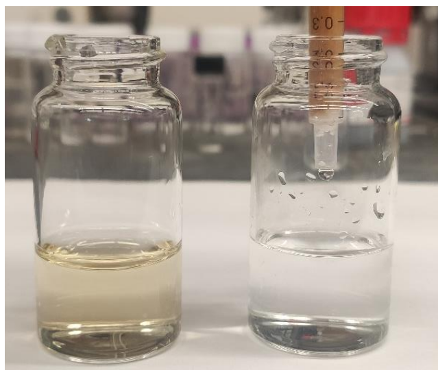
Figure S34. Image of iodine solution (35 mg/L I_2 + 15 mg/L I^- ) before and after through H c OF-7 column.
