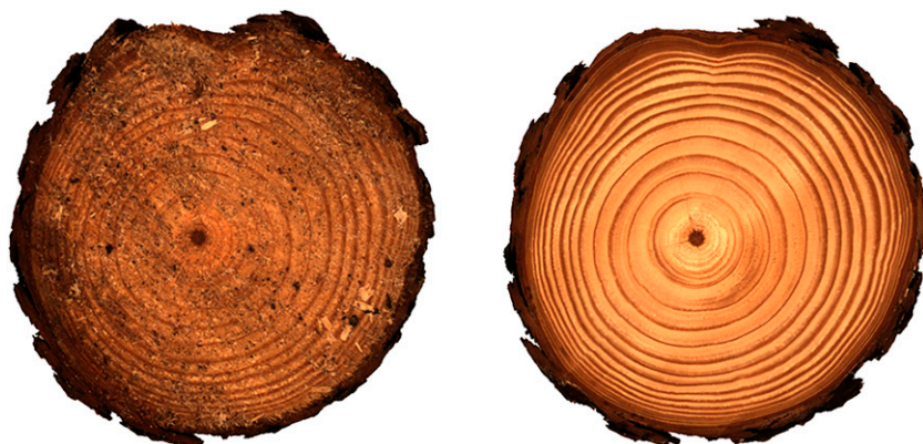
Figure 2. The left image shows the typical surface quality of a chainsaw-cut wood disk; the right image shows the same disk after surface preparation (background removed from both images).
