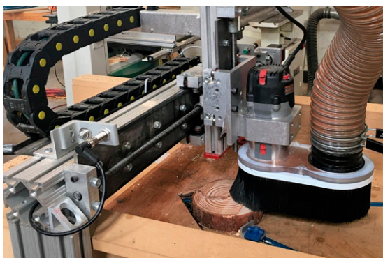
Figure 1. The three-axis computer numerical controlled (CNC) router preparing a cross-sectional disk surface for imaging.
