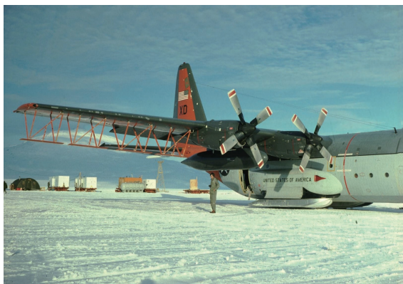
Figure 5 Hercules ski-equipped aircraft (LC-130R) in 1978 with 60 MHz ice radar antennae (comprising four half-wave dipoles) fitted beneath the starboard wing. The 300 MHz antenna is mounted beneath the port wing (unseen).
