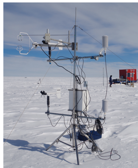
Figure 1 Mobile polar atmospheric parameter measurement system at Taishan Station, on January 11, 2014. Micro-thermal sensors are ~2.0 m above the snow surface.
