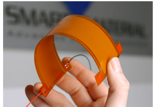
Figure 5.13: Flexibility test of an MFC by the manufacturer [42]
