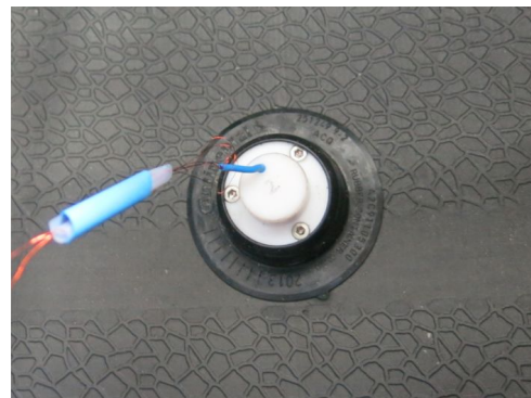
Figure 9.22: Electromagnetic energy harvester embedded in a rubber container, which was glued on the tire inner liner
