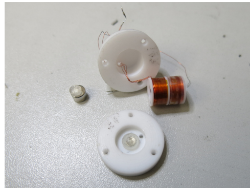
Figure 9.36: Electromagnetic transducer disassembled after testing
