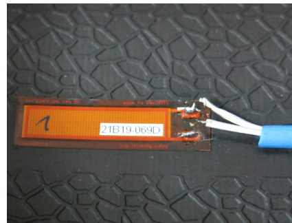
(b) Ruptured wires after testing
