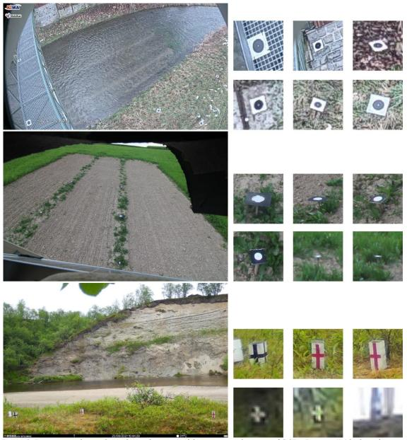
Figure 2. Datasets used to evaluate the performance of the automatic detection of GCPs. Dataset A) Black circles on white background. Dataset B) White circles on black background. Dataset C) Black, red and white crosses on white or black background.
