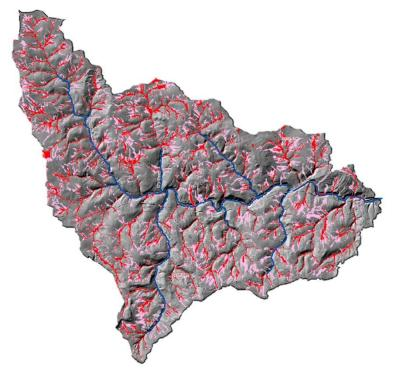
Figure 1. Hydrological connectivity map generated with SCIMAP (https://scimap.org.uk/). Red displays areas which connect most frequently with the floodplain, pink areas show areas that connect frequently, but less often than red (SCI-MAP 2023).
