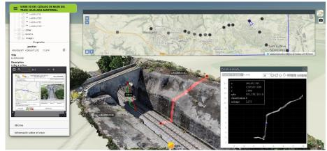
Figure 2. 3D web viewer of the catalog of retaining walls of the Llobregat-Anoia line of FGC, where some of the measurement tools present in the viewer are exemplified and the status of the asset can be consulted.
