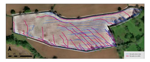
1.84cm/pix resolution drone data from DJI Phantom 4 RTK (blue) in Herefordshire, UK. The drone orthophoto is overlaid on the base map sourced from Mapbox (SCALGO Live 2023).
