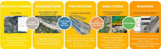
Figure 1: Workflow and results obtained when applying UAV to geotechnical assets in railways.
