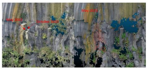
Figure 2. Example of change detection with UAV Photogrammetry comparing three campaigns.
