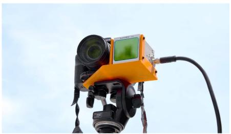
Figure 1: Livox Avia and DSLR camera equipment.
