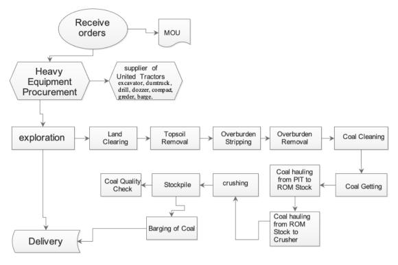
Fig. 2 - Coal Production Process Flow
