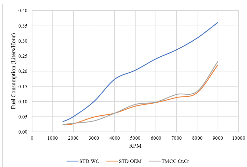
Fig. 3. Trends in fuel consumption at each rpm
