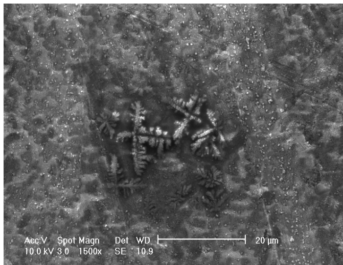
Fig. 3. SEM image of Cerastat sample. Note that the contrast in this figure is dominated by electron yield rather than charging.
