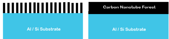
Figure 2. Idealized cross-section diagrams of the Pillar Model (left) and the multilayer model (right). Electrons would approach the sample from the top-down during electron yield testing.
