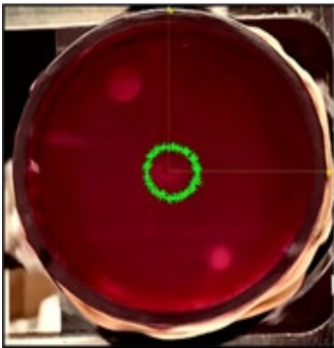
Fig 3 Microcarrier bead cluster tracking inside the media using Pasco Capstone™ software.
