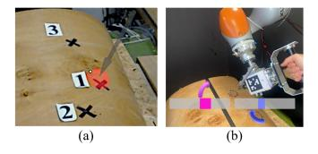
Fig. 5. The visual feedback displayed to the user by the augmented reality (AR) interface under (a) haptic guidance and (b) no haptic guidance
