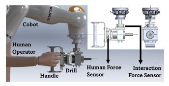
Fig. 2. A closer shot of the hardware components used in our study.
