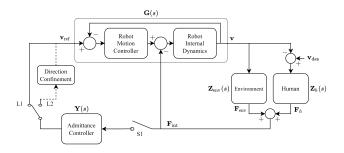
Fig. 3. Closed-loop control system used in our pHRI study.
