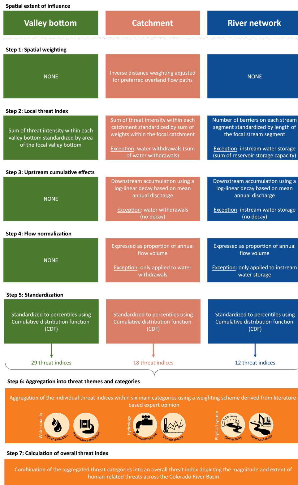
Fig. 2. Schematic diagram illustrating the steps of the workflow for threat index calculations according to the three spatial extents of influence.
