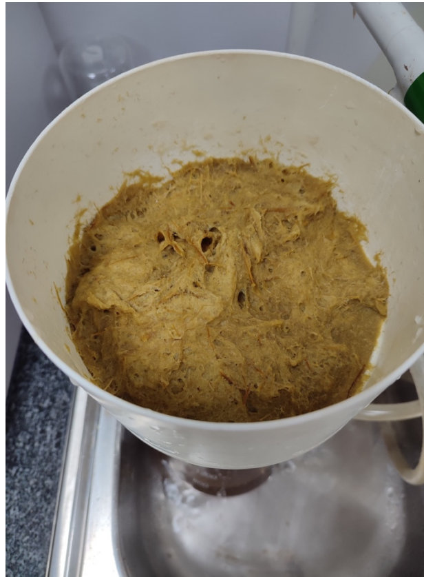
Figure 7. Delignified fibers from Arundo donax .
