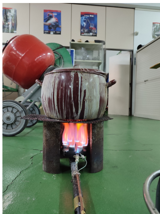
Figure 5. Kraft delignification process developed in the school of Forestry Engineering of the University of Vigo, Galicia.
