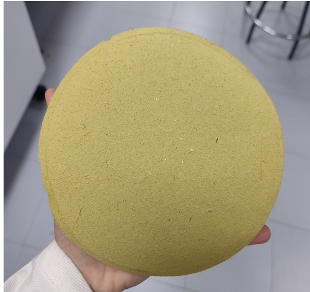
Figure 11. Dry handsheet from Arundo donax leaves.
