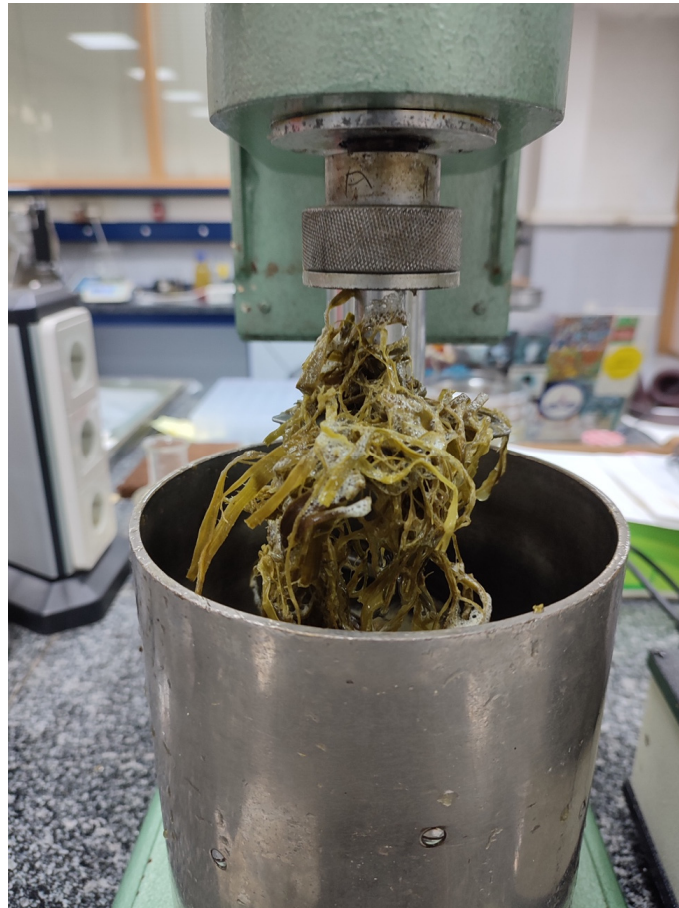
Figure 6. Disintegration process of delignified matter before refining in PFI. Matter from Phytolacca americana stem.
