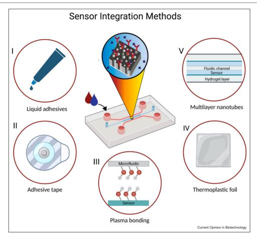
Overview of sensor integration methods recently described in the literature. (I) Liquid adhesive can be used as a bonding agent (utilized in Ref. [5•]), or alternatively, (II) adhesive tape can be employed (utilized in Refs. [4,12\*,32,33\*\*,34]). (III) Plasma bonding is often used with PDMS-based microfluidics (utilized in Refs. [30,35]). (IV) Moreover, thermoplastic foil (utilized in Ref. [9]) or (V) multilayer nanotubes (utilized in Ref. [36••]) can be used for sensor integration.
