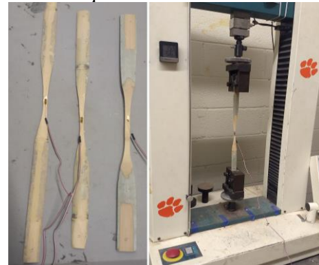
Figure 3: (left) tension test specimens; and (right) setup of tension tests.
