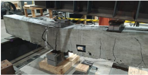
Figure 10: Setup for test and post failure cracks on beam
