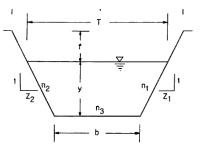
Figure 1. The geometric dimensions for a trapezoidal cross section
