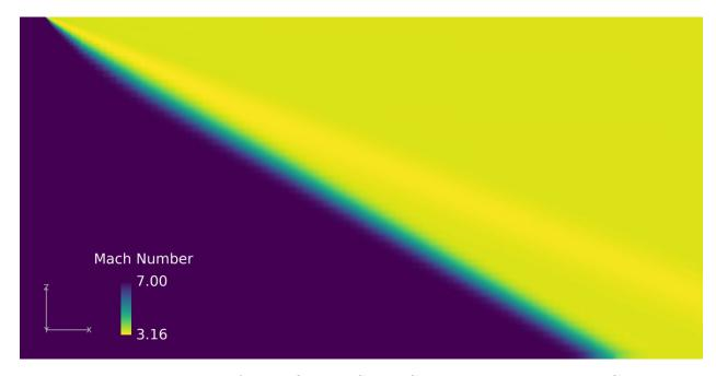
Figure 16: Mach Number for  $30^\circ$  Oblique Shock Created by Top Boundary Condition
