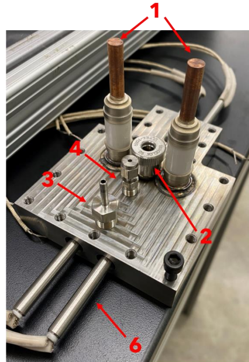
Figure AV-1. Annotated top of the PHPR reactor system. The right side shows the current parts welded onto the assembly. Note: Part 4 has two parts. The figure on the left (CAD) shows the front thermocouple connection, and the right figure shows the back thermocouple.
