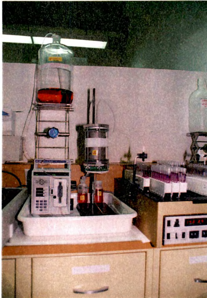
Figure 3. Experimental configuration of laboratory columns. The column was inverted to the in situ position, with the influent entering the bottom of the column, supplied at a constant rate by the medical pump (3M Corporation). Column dimensions were 15 cm in length by 8.5 cm in diameter. Samples of the effluent were collected in the ISCO fraction collector.
