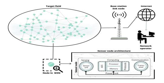
Figure 1 Wireless sensor network (WSN)
