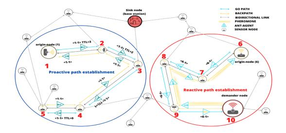
Figure 3 The hybrid mechanism to discover routes in the network
