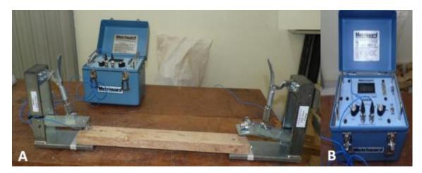
Figure 01: Stress wave timer. A-Sample tested; B-Detail of the equipment
