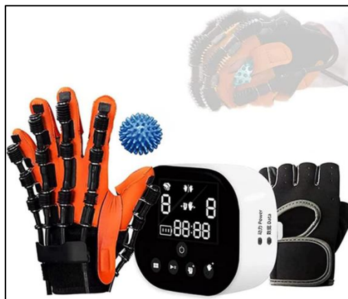
Figure 06: Hand rehabilitation robot glove.
