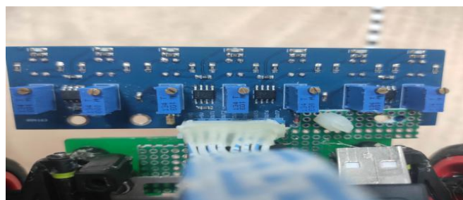
Figure 1 Installation of Greyscale Sensor
