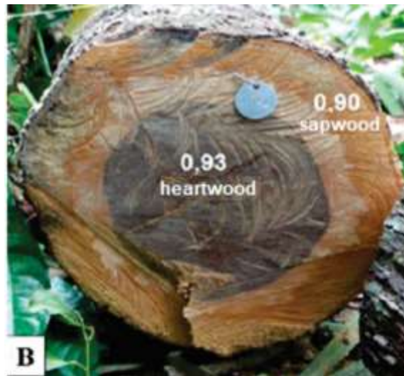
Figure 2. Cross-sectional view of the wood and basic density of the heartwood. Source: Barros, 2016.
