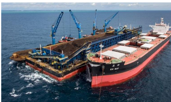
Figure 3. Typical indirect floating transshipment
