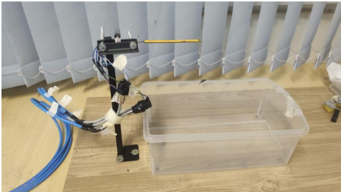
Figure 04. Strain gages connected to the signal conditioning circuit.
