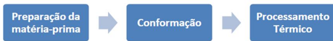
Figure 2 - Basic steps in red ceramic production processes
