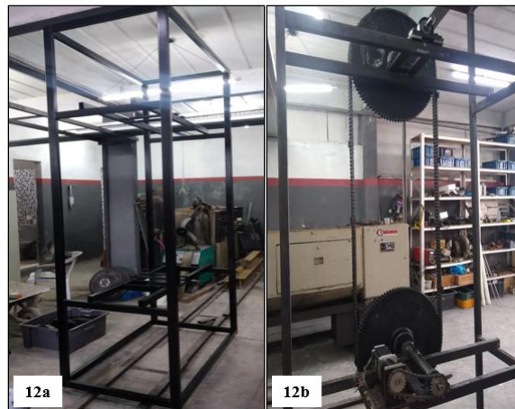
Figure 12. 12a - Elevator structure and 12b - Elevator assembly.
