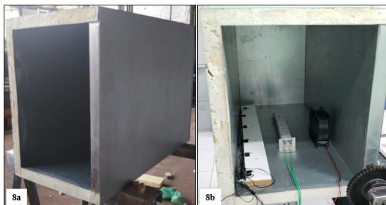
Figure 8. 8a - Thermal insulation module and 8b - Installation of thermal insulation elements.
