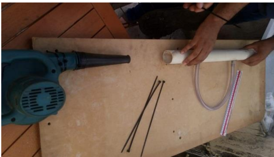
Figure 3 - Pitot Tube being fixed to the MDF board.
