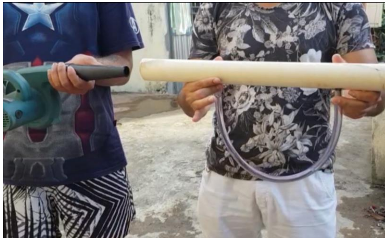
Figure 1 - Pitot Tube experiment with the U-tube inserted and the Makita Ub1103 blower.
