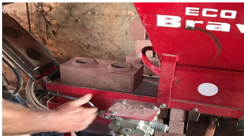
Figure 6- Press for the manufacture of ecological bricks.
