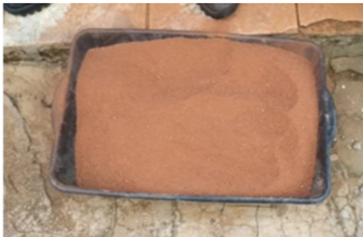
Figure 4- Shards of shredded and sieved tiles
