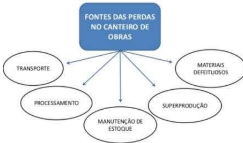
Figure 1- Sources of losses at the construction site
