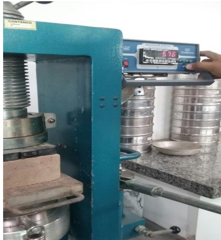
Figure 8- Compression test on ecological brick
