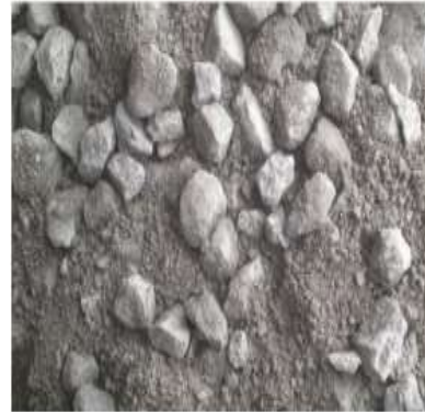
Figure 8: Artificial aggregate. Source: MORAES (2016).
