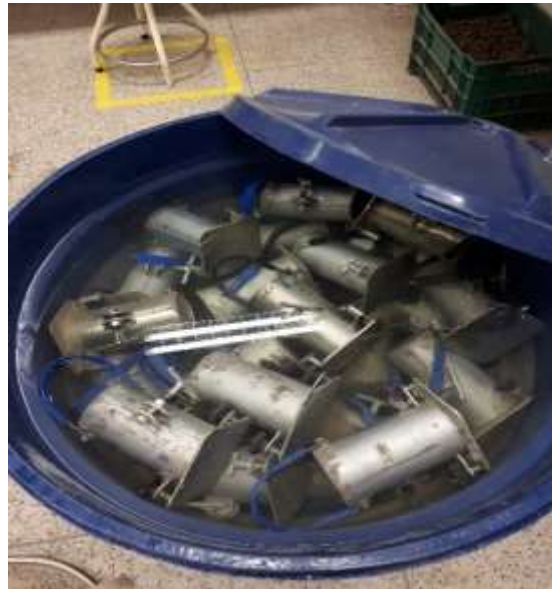
Figure 13: Spicemens submerged in water. Source: AUTHOR (2020).
