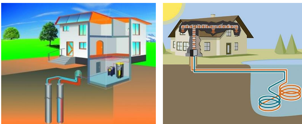
Figure 4 - Vertical Closed Circuit Systems in the Ground and in the Water. Source: Rodríguez (2015) and Geo Journal (2009).
