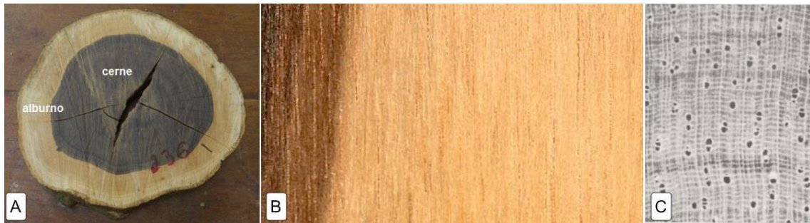
Figure 3. View of the cross section of the trunk (A); contrast between heartwood and sapwood (B); macroscopic aspect in cross section (C).
