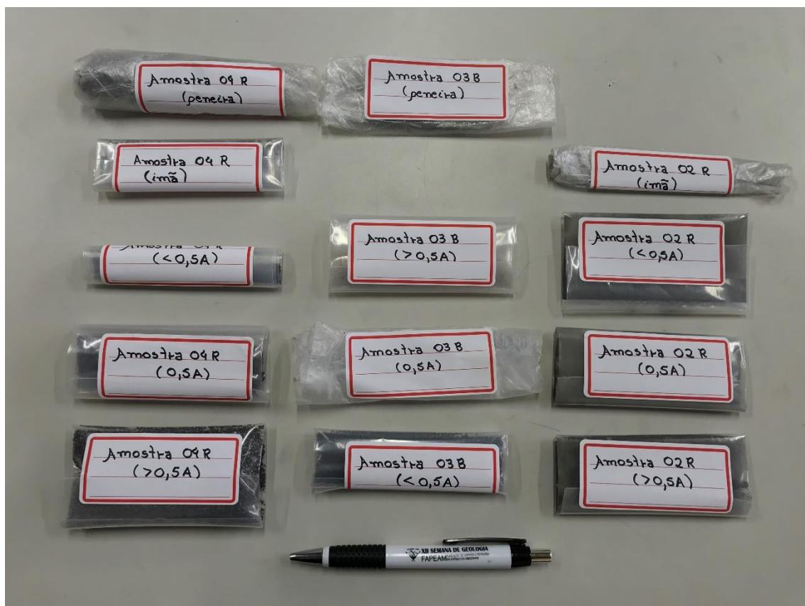
Figure 3. Samples already separated by the FRANTZ Magnetic Separator.
