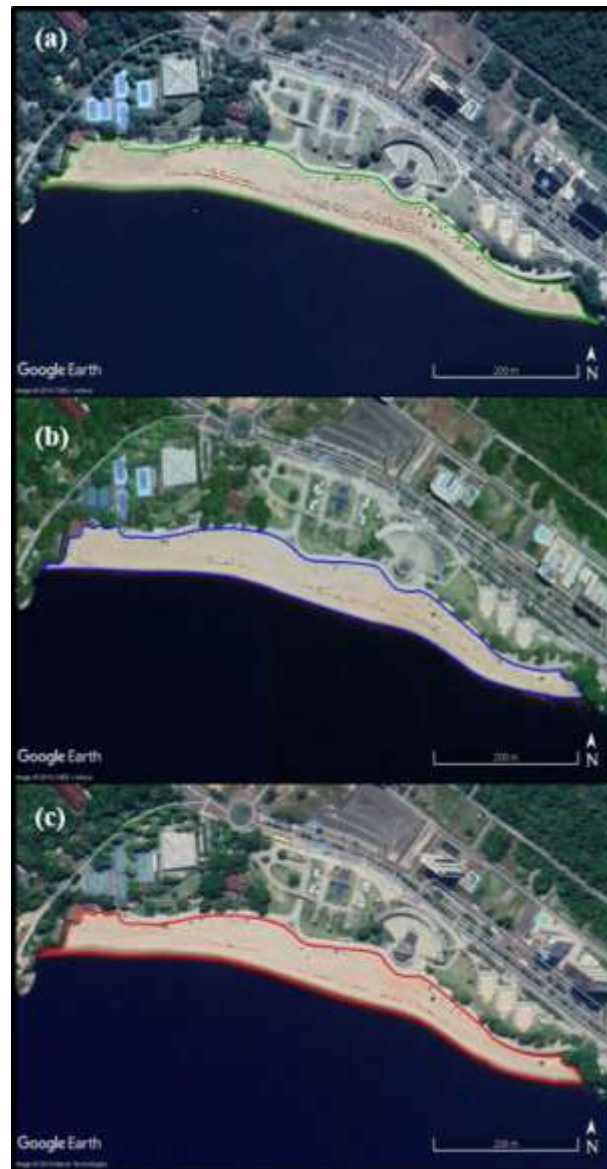
Figure 18: A) Flood on 7/29/2017, elevation: 27.69 m; B) Flood on 07/20/2018, elevation: 28.15 m; C) Flood on 7/31/2019, elevation: 28.34 m. The polygons in each image were used for area calculations. Source: Images taken in the Google Earth Pro program and elevations data taken from the Porto de Manaus website.
