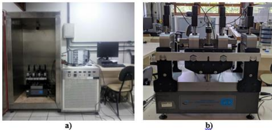
Figure 3. a) climate camera; b) 4-point test apparatus for complex module assay
