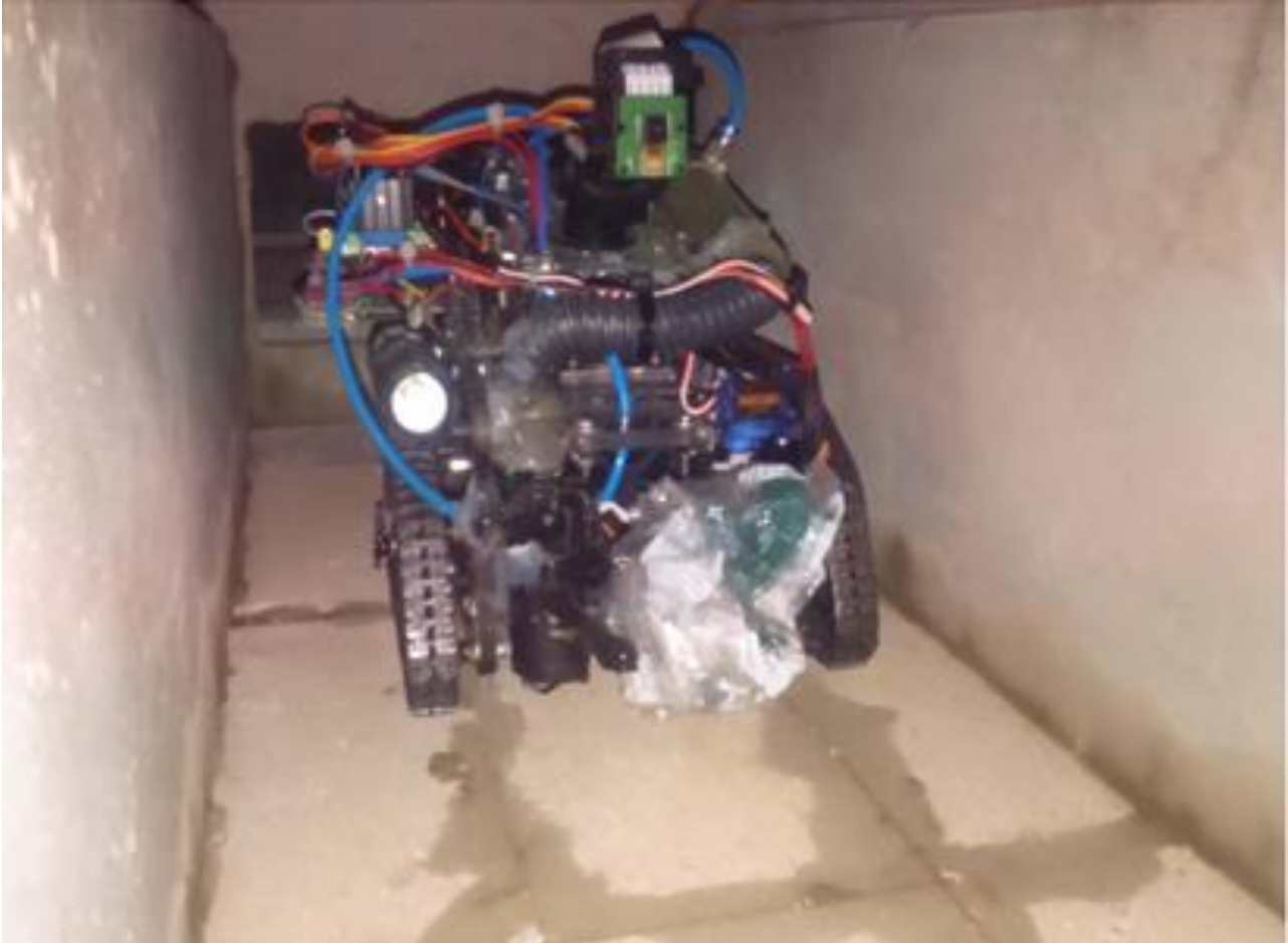
Figure 5. Locomotion by mats in a duct.
