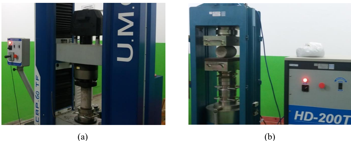
Figure 4 - (a) Axial compression strength test and (b) diametral compression traction
