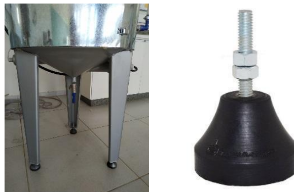
Figure 8. Tripods and dampers for controlling vibrations.
