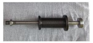
Figure 7 - Interchangeable withdrawal shaft Source: Author
