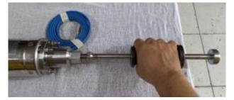
Figure 11 - Tool Kit Coupled to Pump Motor Cover Source: Author
