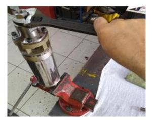
Figure 14 –Drive Fixed Pump for Unscrewing Plastic Part Source: Author
