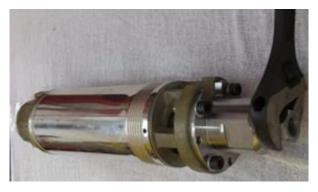
Figure 13 - Hexagonal Center Flange Coupled to Pump Source: Author
