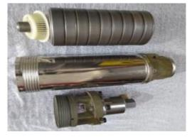
Figure 15 - Disassembled Pump
