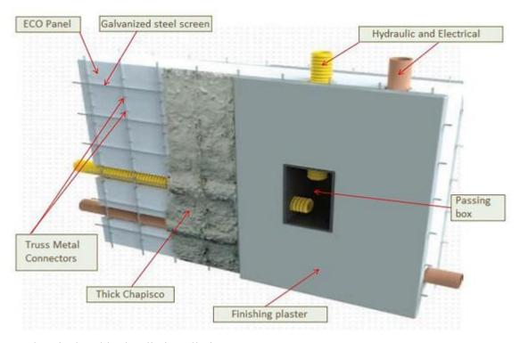
Figure 04: Electrical and hydraulic installations
