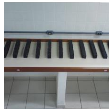
Figure 10. Beams ready for Fatigue Testing
