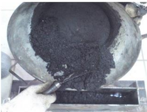
Figure 9. Inserting Asphalt Mix into Mold
