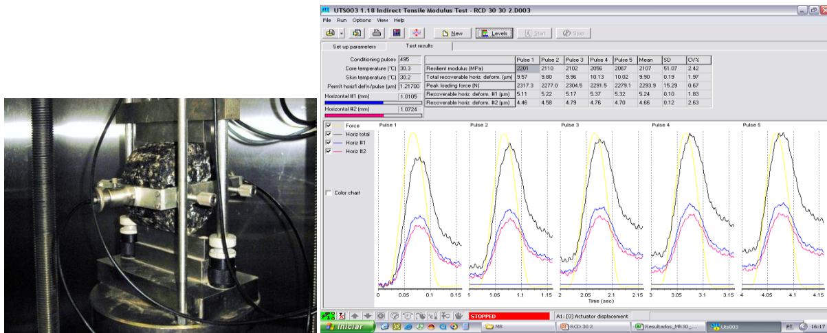
Figure 2 - UTM specimen press with MR assay graphical interface.
