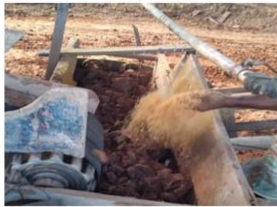
Figure 8: Mixing with water and sawdust.
