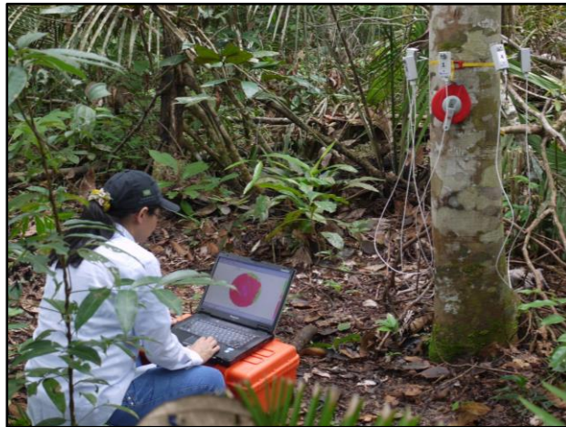
Figure 2: Application of the pulse tomograph to the tree stem.
