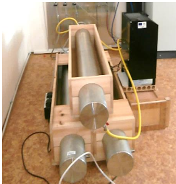
Figure 5. Cooling the metal hydride tank with a water cooler.
