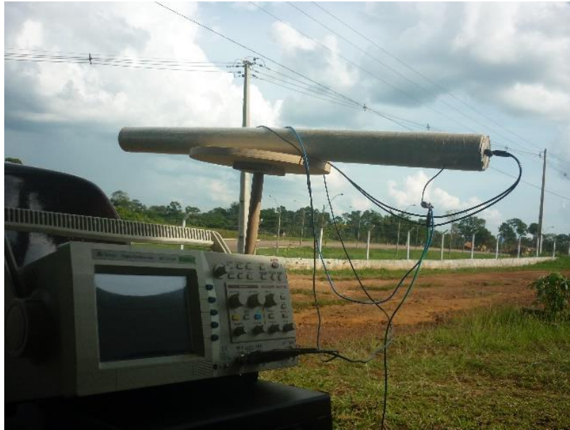
Figure 6. Prototype placed in front of 13.8 kV distribution line.
