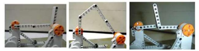
Figure 3. Some singularity configurations of 5R mechanism built with LEGO.
