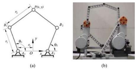
Figure 2. (a) Parameters of the 5R Mechanism; (b) Prototype assembled with LEGO.
